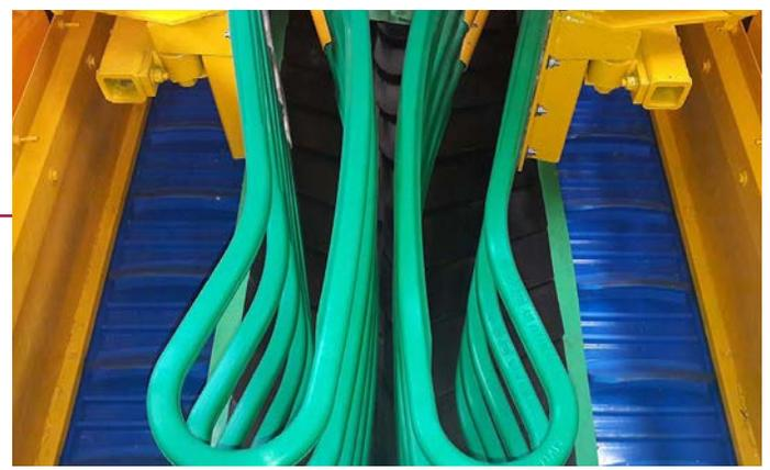
For optimum results most grape-harvesting machines choose to immobilise grapevines during the shaking process, avoiding risk of damage by friction between the grapevines and the grape-harvesting machine that take them directly to hoppers.
